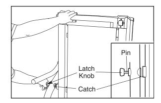
Hold the treadmill firmly with both hands, and lower the frame to the floor. Do not drop the frame to the floor. CAUTION: To decrease the possibility of injury, bend your legs and keep your back straight.
